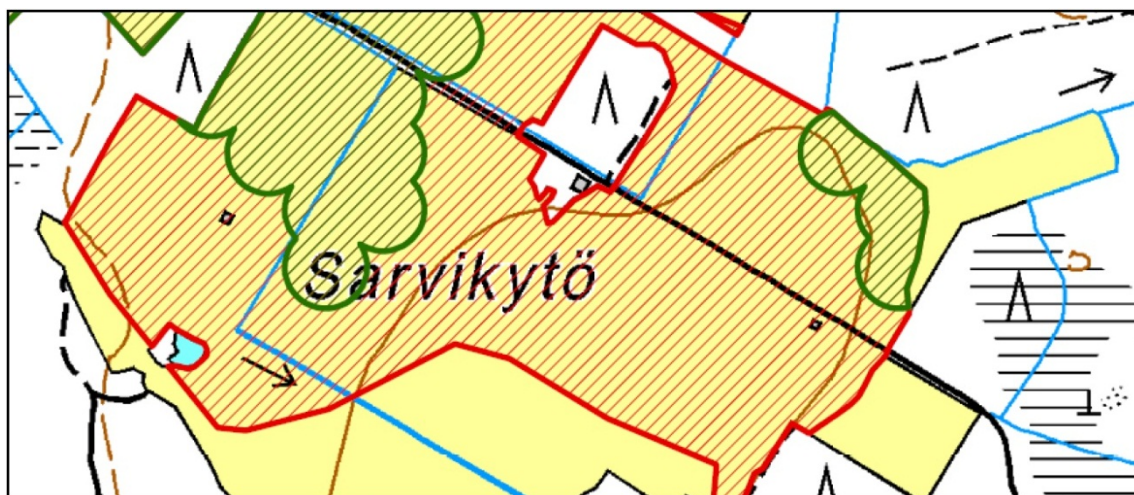
Fig. 1. An example of the GIS-analyse. Peatland according to soil maps are marked with red. The area where low gamma radiation intensity indicates deep peat is marked with green. There is a basic map in the background, in which agricultural fields are marked with yellow colour.
