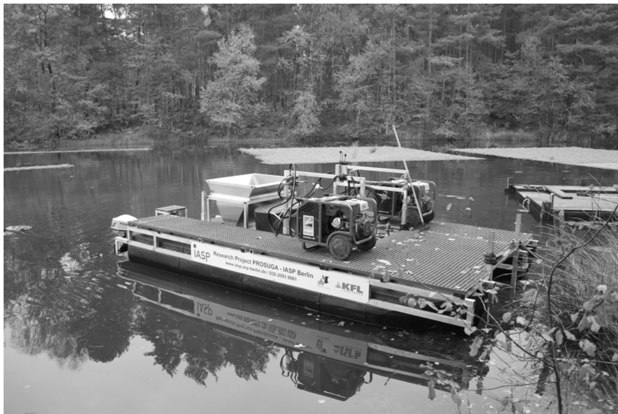
Fig.2. Harvester catamaran developed.
