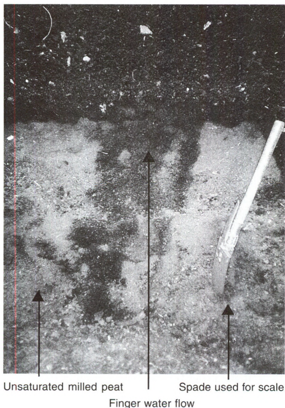
Fig. 1: Finger storage associated with bypass flow in a field stockpile
