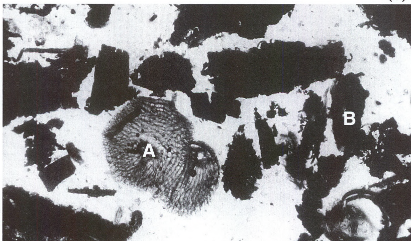
Fig. 6: Photomicrograph of stained Sphagnum moss fragments (A) and amorphous particles (B) to illustrate the difference in the nature of the staining process.
