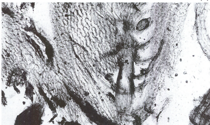
Fig. 5: A photomicrograph under plane polarised light of a Sphagnum moss fragment exhibiting a cellular internal structure from Noggusboy milled peat stockpile.
