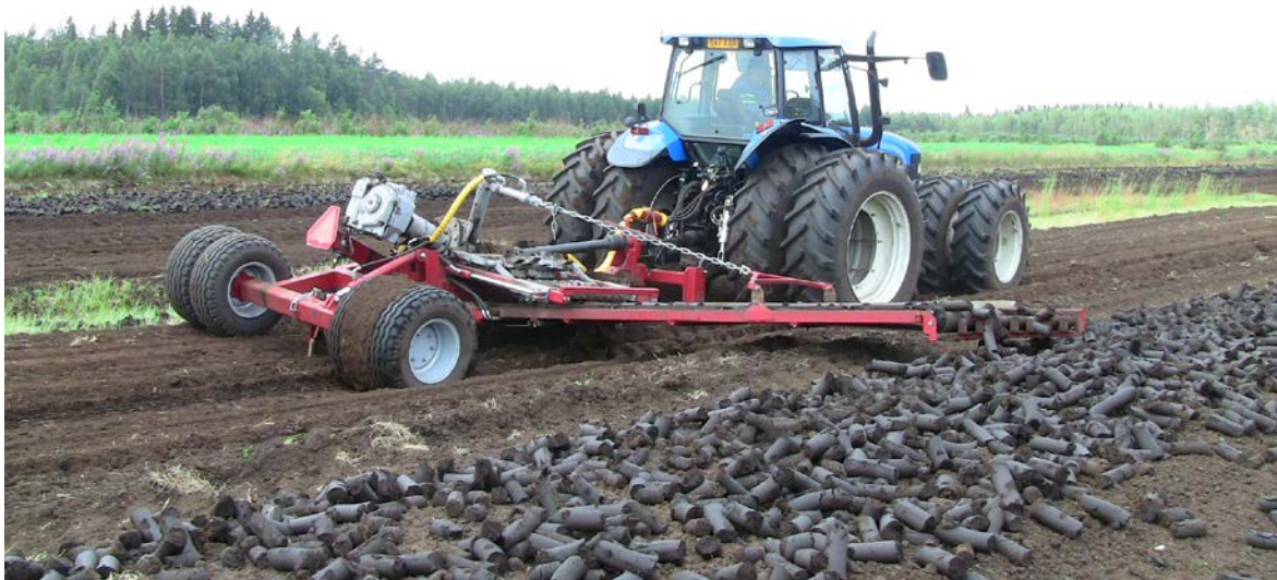
Figure 1. Sod peat cutting machine developed for Multi-Layer method.
