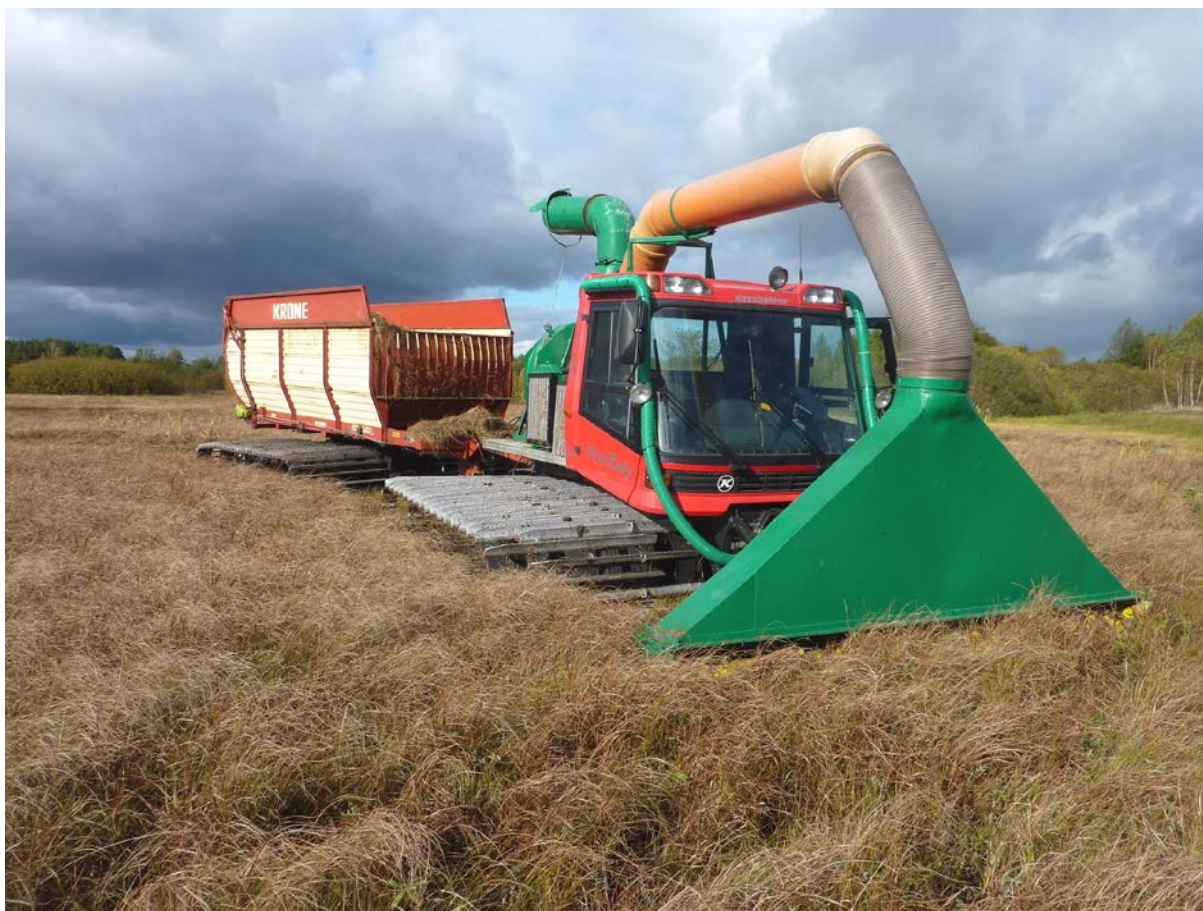
Fig. 2. Modified snow groomers for harvesting peatland biomass. Left: mulching and collecting biomass in a single process step in Belarus (W. Wichtmann). Right: Chopping and collecting biomass in Germany in a second step after mowing and setting in a swath (C. Schröder).
