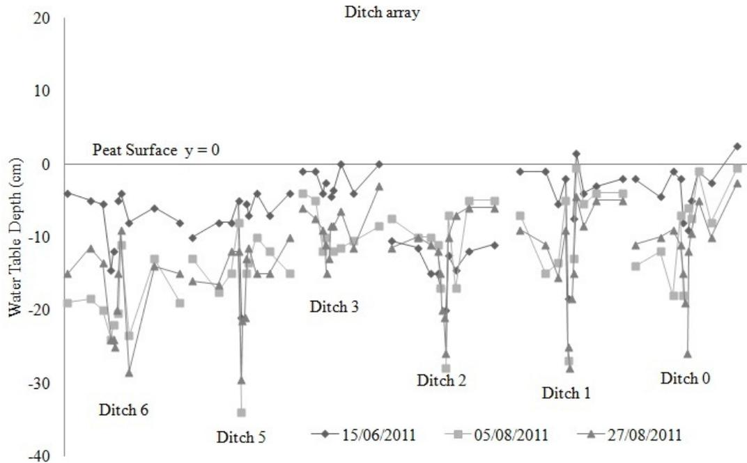
Fig. 2. Water table depths in ditch array from manual measurements taken during months of June and August 2011 of dip-wells placed 0.5, 1, 2, 5, 10 and 20 metres each side of each drain. The x-axis scale is set to scale for dip-well position across a single ditch but is not accurate between ditches.
