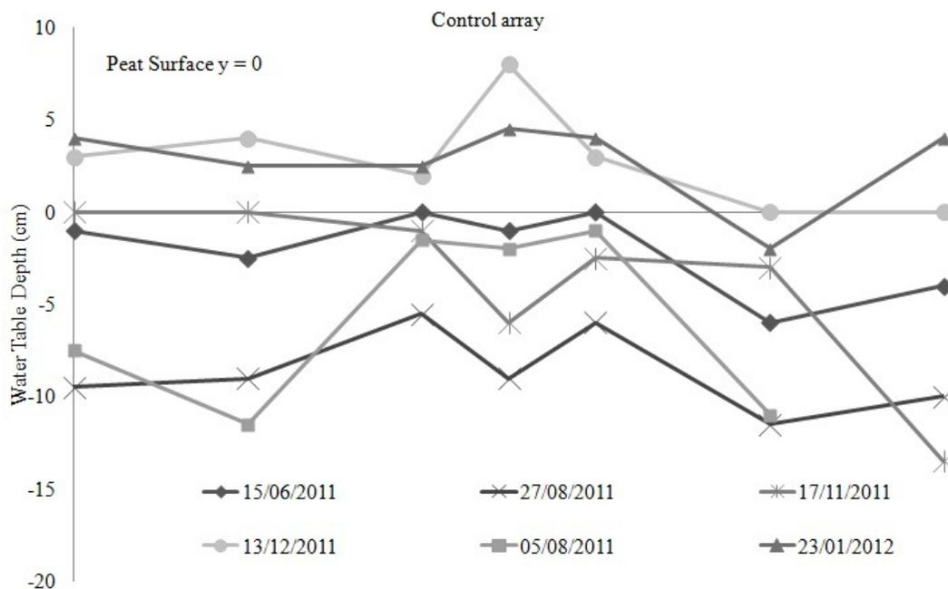
Fig. 4. Water table depths in control array from manual measurements taken during months of June 2011 through to January 2012, of dip-wells placed 0.5, 1, 2, 5, 10 and 20 metres each side of each drain. Dip-wells within control array are set 10 metres apart.
