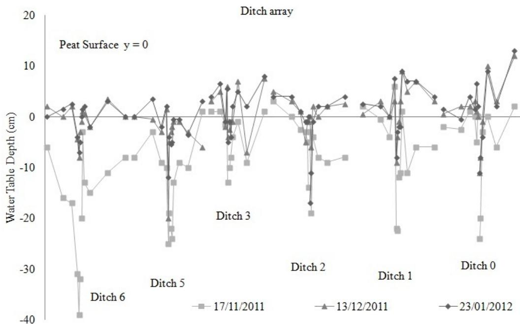
Fig. 3. Water table depths in ditch array from manual measurements taken during months of November and December 2011 and January 2012, of dip-wells placed 0.5, 1, 2, 5, 10 and 20 metres each side of each drain. The x-axis scale is set to scale for dip-well position across a single ditch but is not accurate between ditches.
