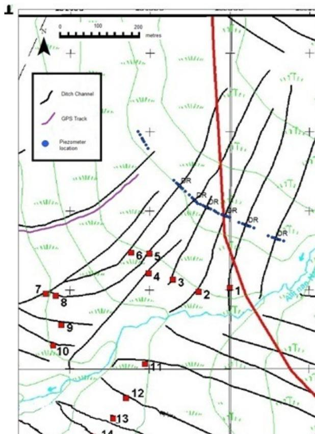
Fig. 1. Map of ditch blocking site, Gordonbush estate. Although there is a ditch marked close to the control array site, blue points further left, it is completely in-filled and our mapping of clear drainage is identified by the purple line. Therefore, we still feel that the control array dip-well positions are not affected by ditch drainage.
