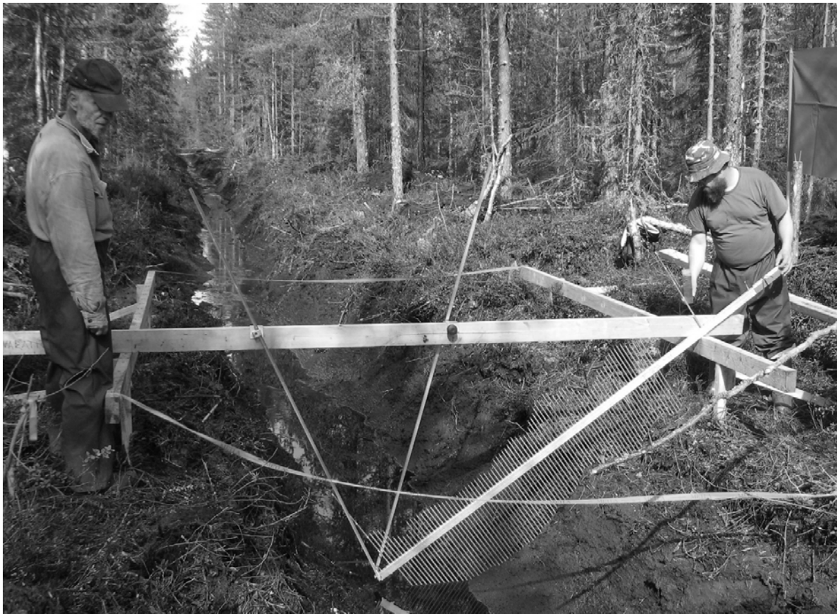
Fig. 2. Pin meter measurement setup.
