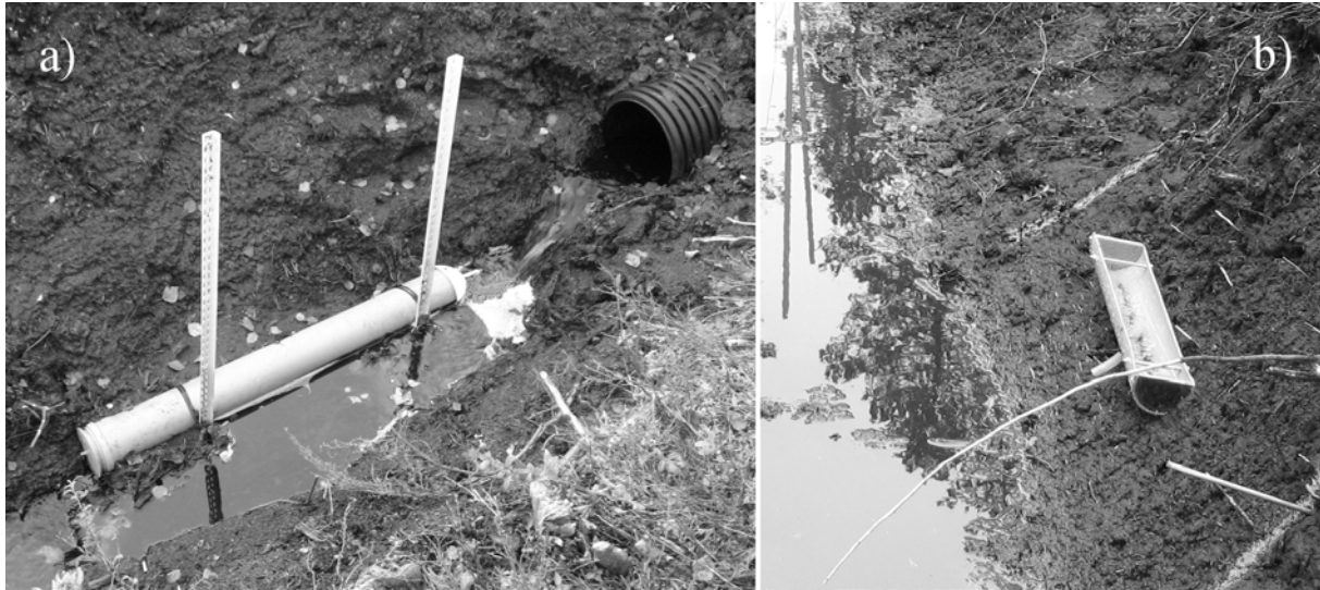
Fig. 3. TIMS-collector for suspended sediment (a) and ditch sidewall collector for eroded soil (b).
