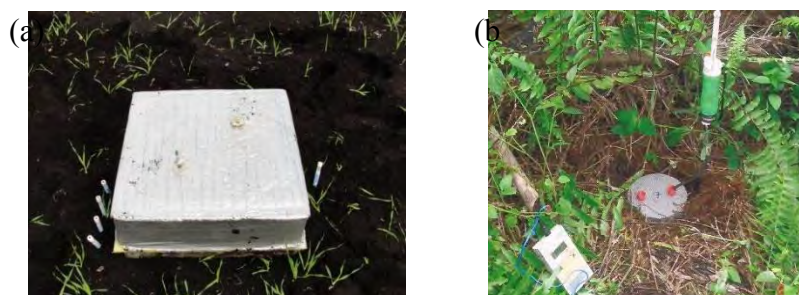
Figure 1: Method of gas collection. (a) Non-steady state chamber design under vegetable production, and (b) Close chamber design under pineapple and oil palm plantation.
