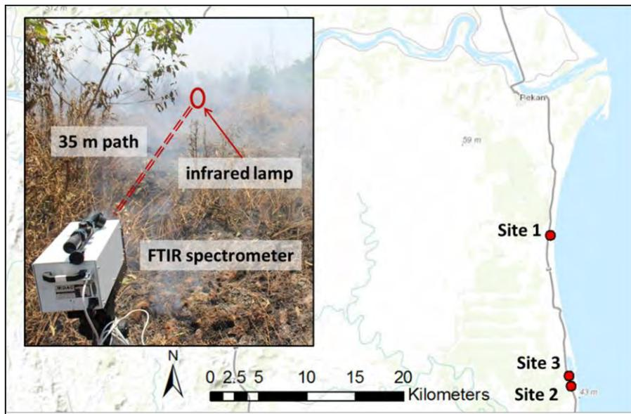
Figure 2: Map with location of three burn sites south of Pekan (see Table 2); (inset) photograph of a typical OP-FTIR setup at Site 2 using a 35 m path between the FTIR spectrometer and infrared lamp.
