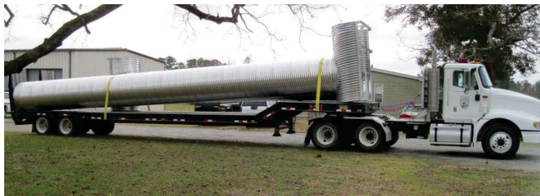
Figure 2: Pre-fabricated aluminum water control structure ready for transportation to installation site. Culvert diameter: 1.2 m. Culvert length: 14 m. Riser height: 2.1 m.
