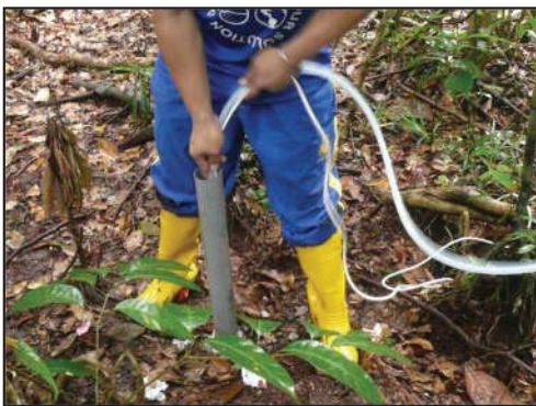
Figure 5: Inserting the water pump instrument into borehole casing.
