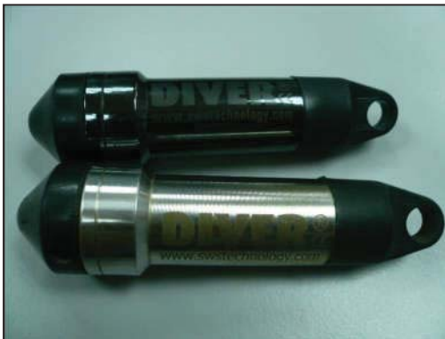
Figure 2: Mini diver (above) and Cera Diver (below) used in the water quantity study.
