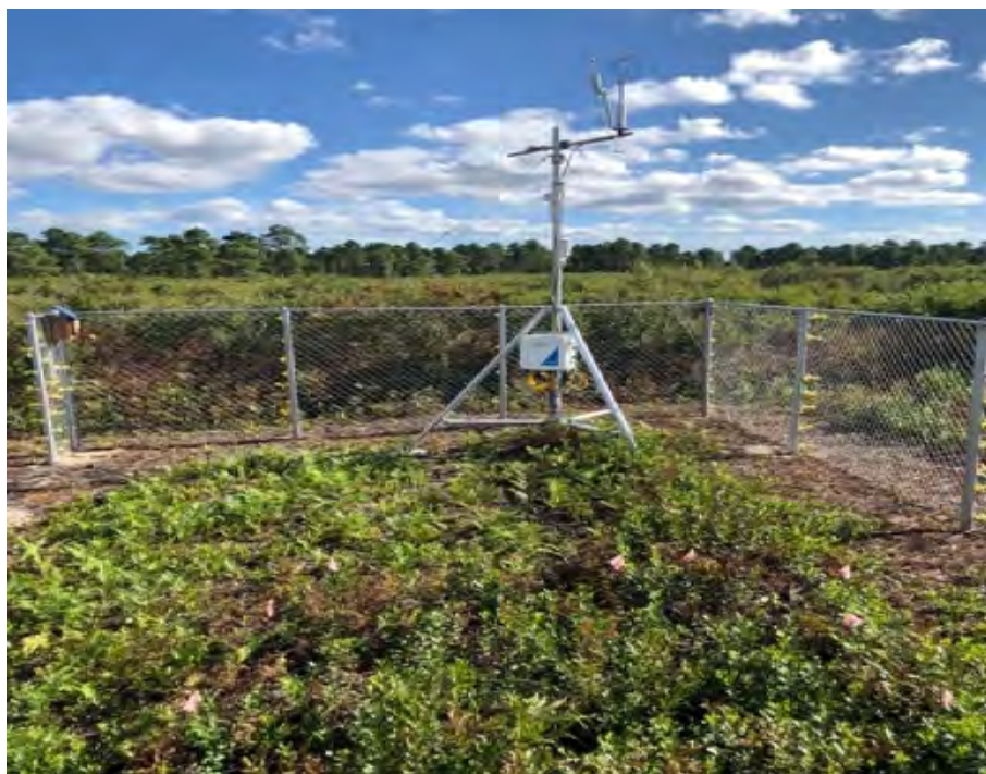
Figure 2: An eddy flux tower in a pocosin shrub bog site in Hyde county North Carolina used to measure carbon dioxide gas losses and storage in peatlands. An electric fence was erected to deter wildlife destruction or disturbance.
